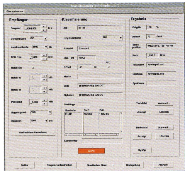
FIG 1 Example of a result window for classification results, signal parameters and receiver settings (status)
